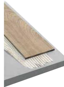
This is the traditional installation method: the geometric shapes are glued with a special adhesive to a thoroughly prepared surface or underfloor that is hard, dry and flawless.
